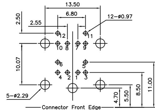
RECOMMENDED P.C.B LAYOUT(PCB THICKNESS: 1.6mm)
